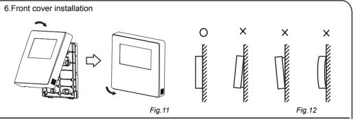
After adjusting the front cover and then buckle the front cover; avoid clamping the communication switching wire during
