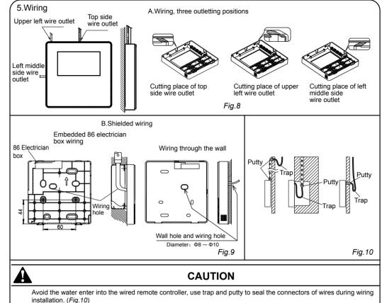
When under installation, reserve certain length of the connecting wire for convenient to take down the wired remote controller while during maintenance.
