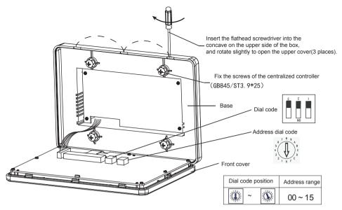
Fig. 1.2 Installation diagram
