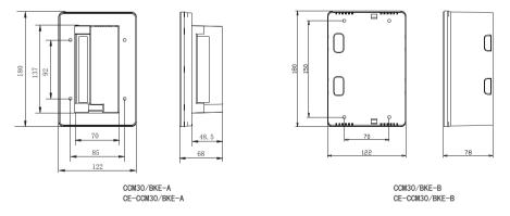
Fig.1.1 Centralized controller size (unit: mm)
