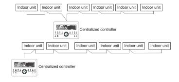
Fig.1.5 Wiring diagram of centralized controller and indoor unit of air conditioner
