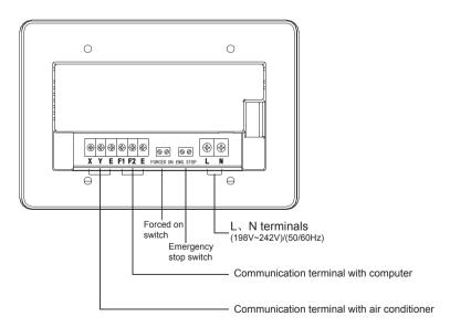
Fig.1.3 Terminal instruction of centralized controller
